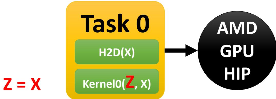
**Z:** RAW dependency b/w Task 0 (GPU) and Task 1 (CPU)
